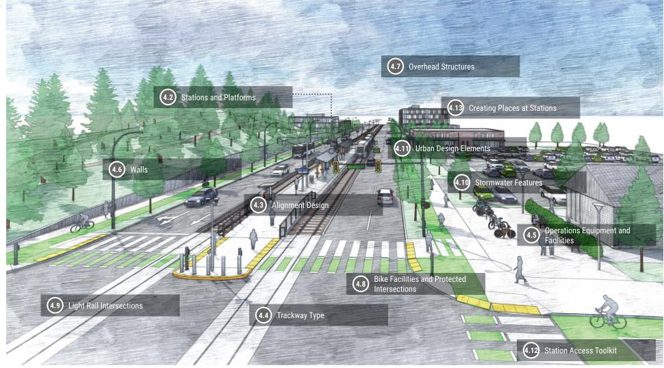
Figure 4.1: Typical Design Elements within a Station Area (this illustration is not representative of any location along the Southwest Corridor Light Rail Project)
