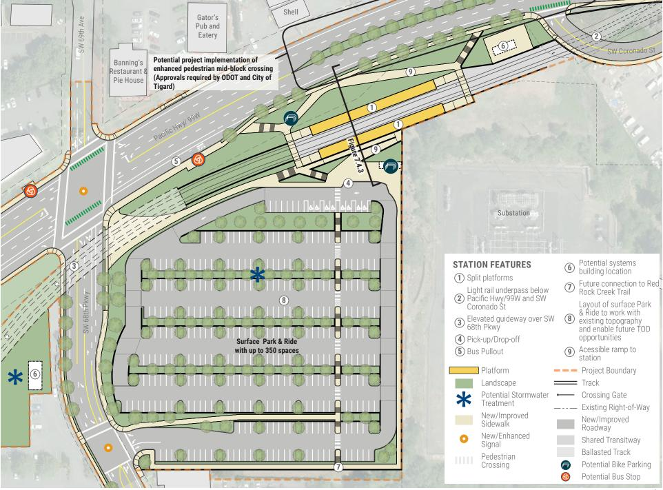
Figure 7.4.4 DRAFT 68th Parkway Station Plan; Design is conceptual and will be further developed through community engagement and technical design efforts
