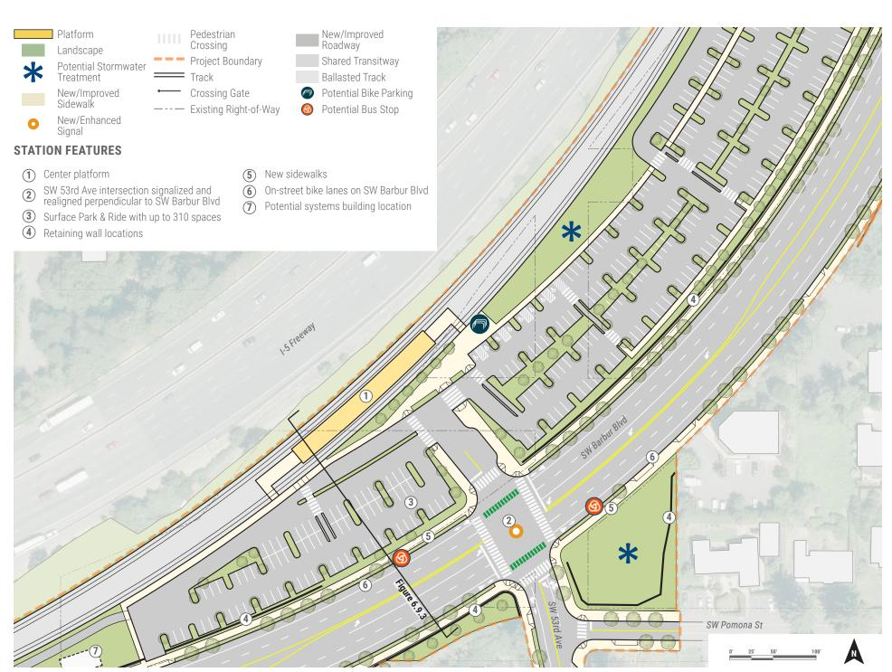
Figure 6.9.4 DRAFT 53rd Station Plan; Design is conceptual and will be further developed through community engagement and technical design efforts
