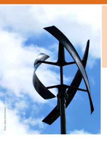
Vertical-axis wind turbines (VAWTs) offer several advantages over traditional, horizontal-axis wind turbines (HAWTs). VAWTs are highly efficient and do not require as much wind to generate power, allowing them to be closer to the ground where wind speed is lower and where they can be maintained in safer and more efficient ways. They are also omni-directional, meaning they do not have to point into the wind, eliminating the need for wind-sensing and orientation equipment.
